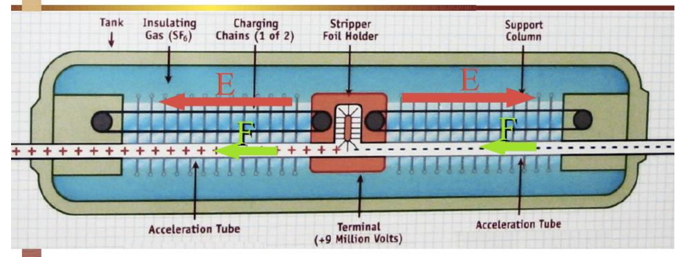
Tandem Van-de-Graaf accelerator E=1.8 MV / m
